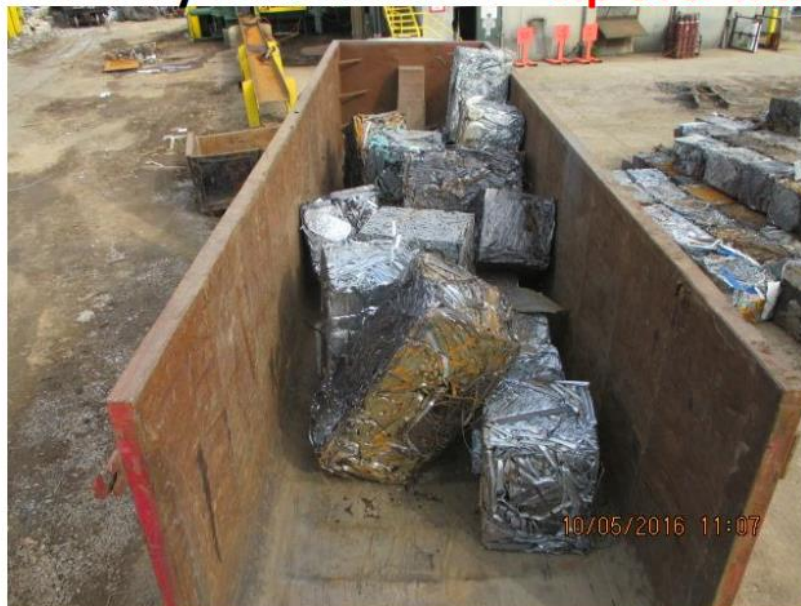
Unevenly loaded trailer – Tip over Risk
